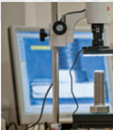
Microscope de mesure Hitec Hitec- Measuring microscope
